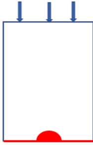
Figure 13. Beam with surface-breaking crack: yz plane
